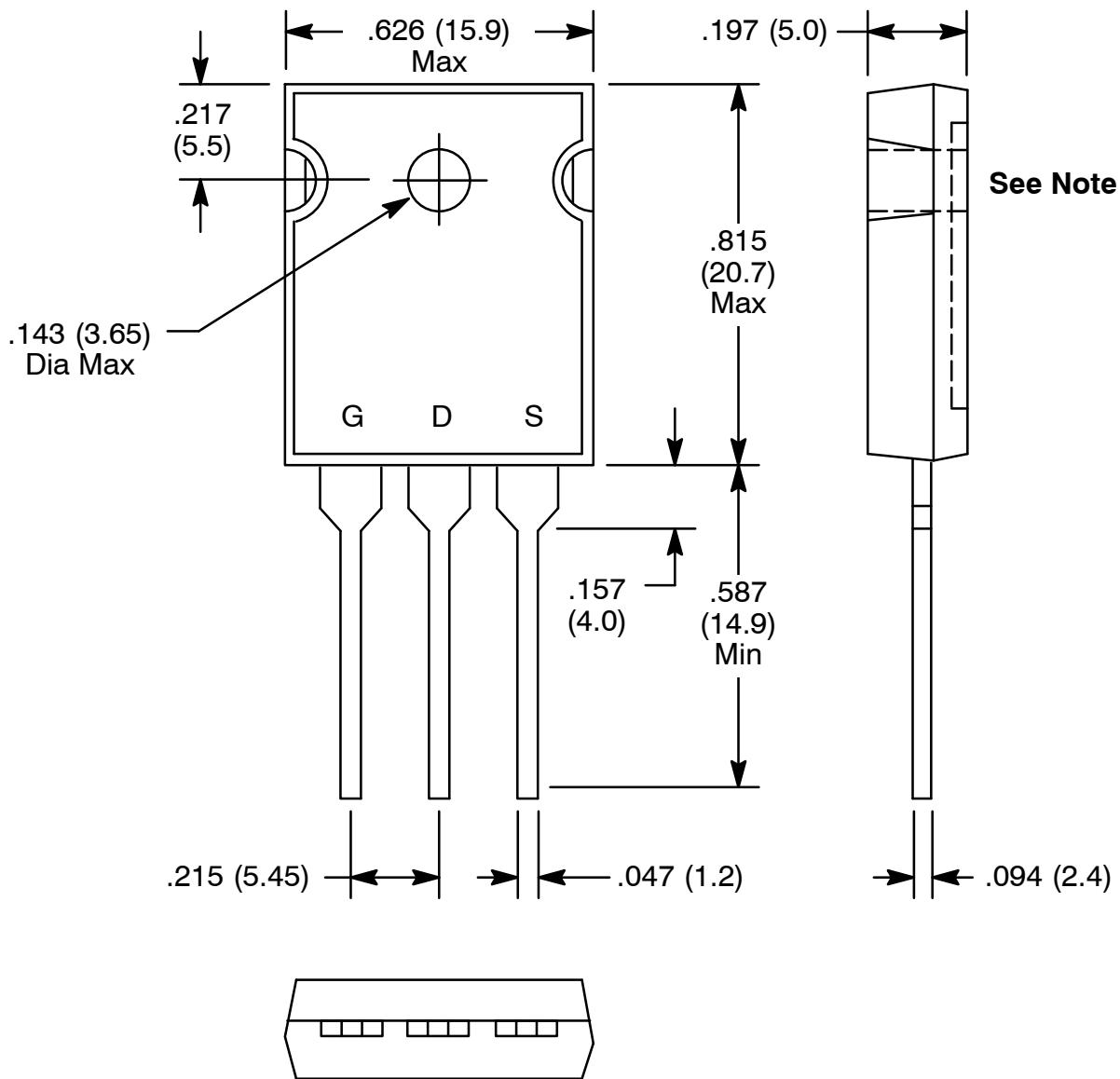
**Note:** Pin 2 connected to metal part of mounting surface.
