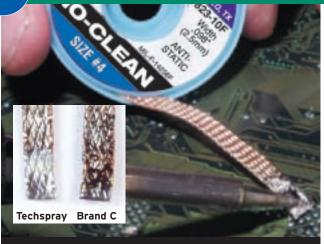
Quickly removes solder without leaving harmful residues.
